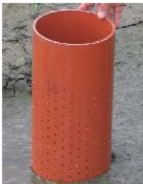
Field water tube from PVC Note the holes on all sides
